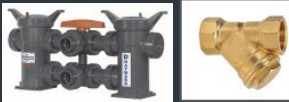
Duplex basket strainers (strainer mesh must be smaller than spray jet orifice) or 'Y' strainer (PSF Equipment)
