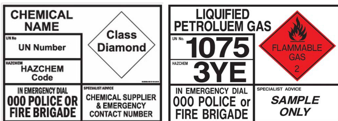
Figure 13.2 Template for a placard for a hazardous chemical stored in bulk
