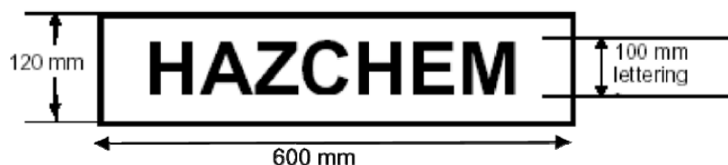
Figure 13.1 Form and dimensions of outer warning placard
